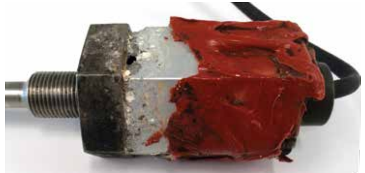
Standard aluminum-housing position sensor destroyed by exposure to acidic water near a scale cracker in a steel rolling mill.
