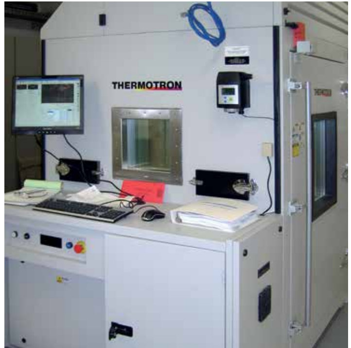
HALT testing chamber and data logging equipment.
