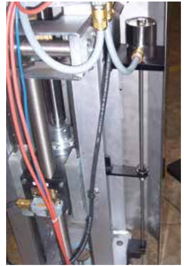
Externally mounted cylinder position sensor used to provide signal redundancy.
