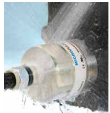
Hermetically-welded sensor housing rated to IP69K. Shown with cable protection system installed to prevent cable damage and subsequent liquid ingress via the cable entry.
