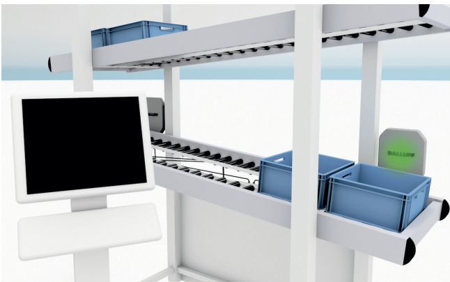
HF or UHF readers detect containers equipped with data carriers in the kanban shelving
